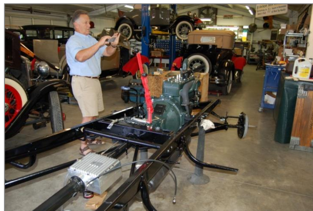
~ 9 ~ Mitchell synchronized transmission and overdrive
