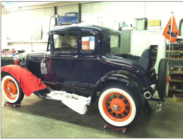
August 2014 – body & tires go back on the frame
